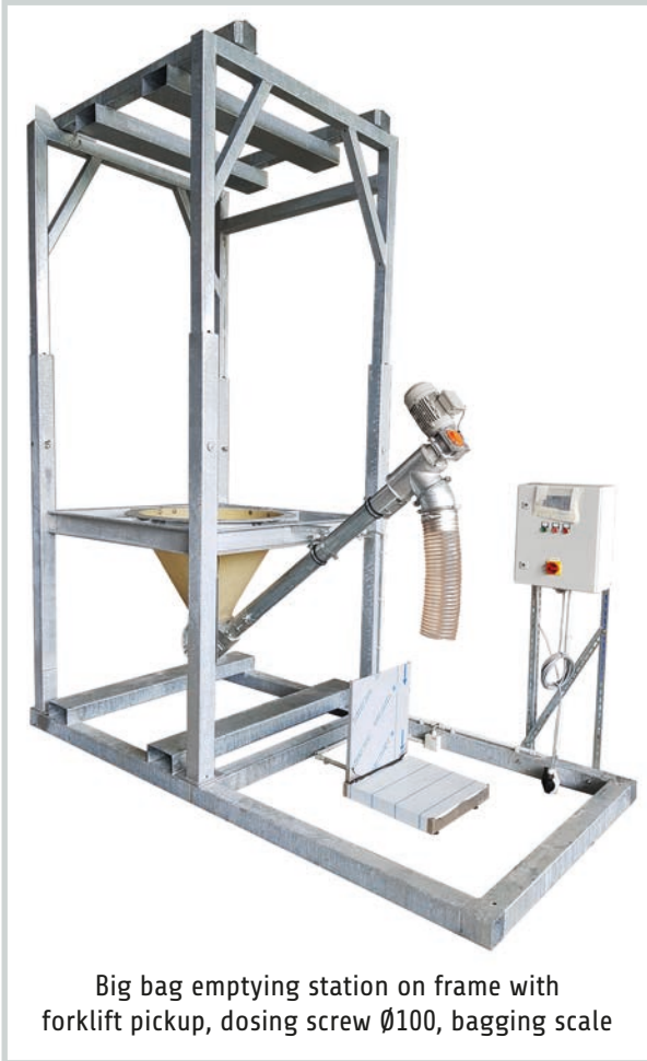
Big bag emptying stations with screw discharge for feeding a vertical mixer
