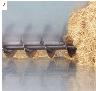
2 Screw conveyor in the buffer tank
