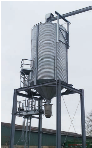
Loading silo 64 m 3
