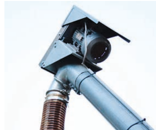
Drive station with rain cover
