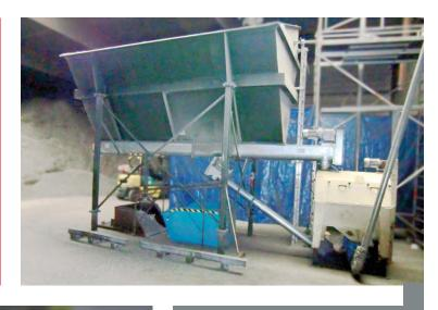
Mobile belt conveyor with big receiving hopper for gentle conveying
