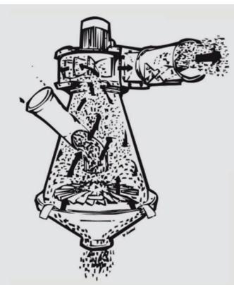
The Kessens Precleaner operates on the principle of air classifier. All lightweight components are thoroughly vacuumed. The extracted dust- air mixture is purified via a cyclone.
